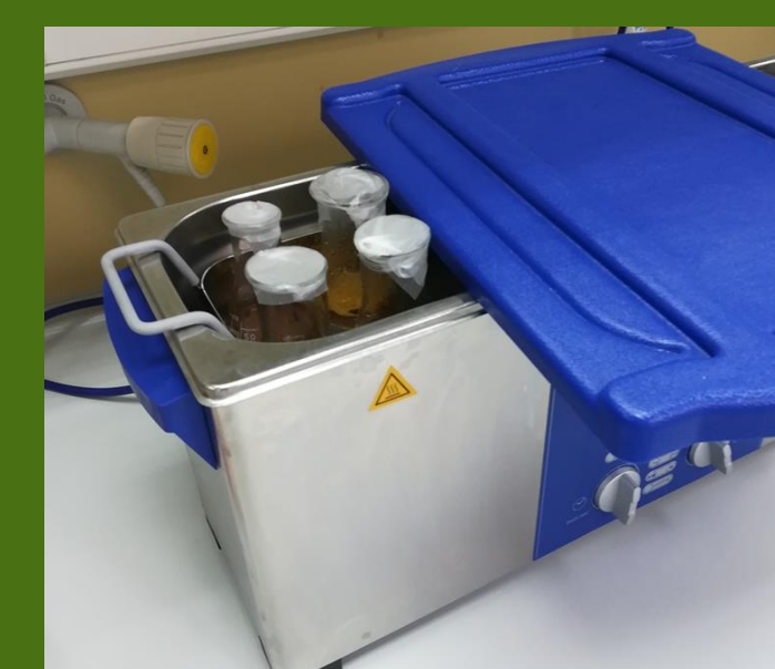
Fig.3 Ultrasound-assisted extraction of tobacco waste
