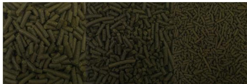
Screw pressed cake (nozzle ID 12, 9 and 6 mm)
