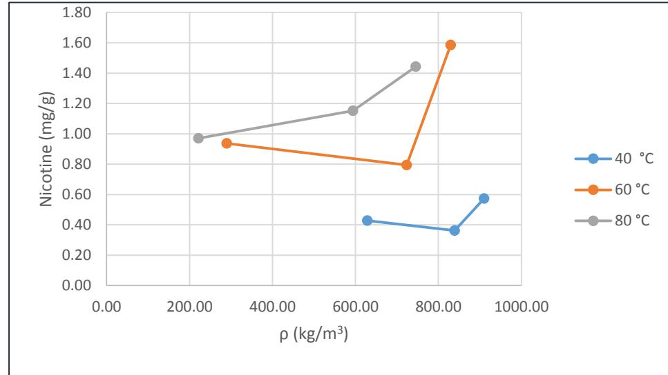
**Figure 4:** Nicotine content of tobacco waste vs. solvent density ( $\rho$ ) at different temperatures during SC-CO<sub>2</sub> extraction
