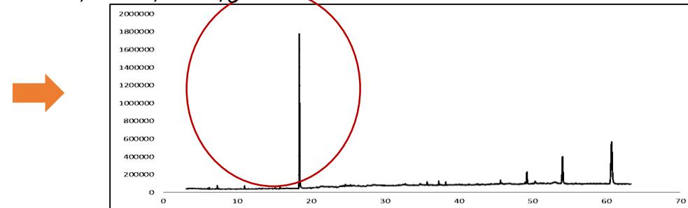
Figure 2: GC-MS midrib chromatogram obtained under UAE condition of 70 °C, 30 min, 30 mL/g
