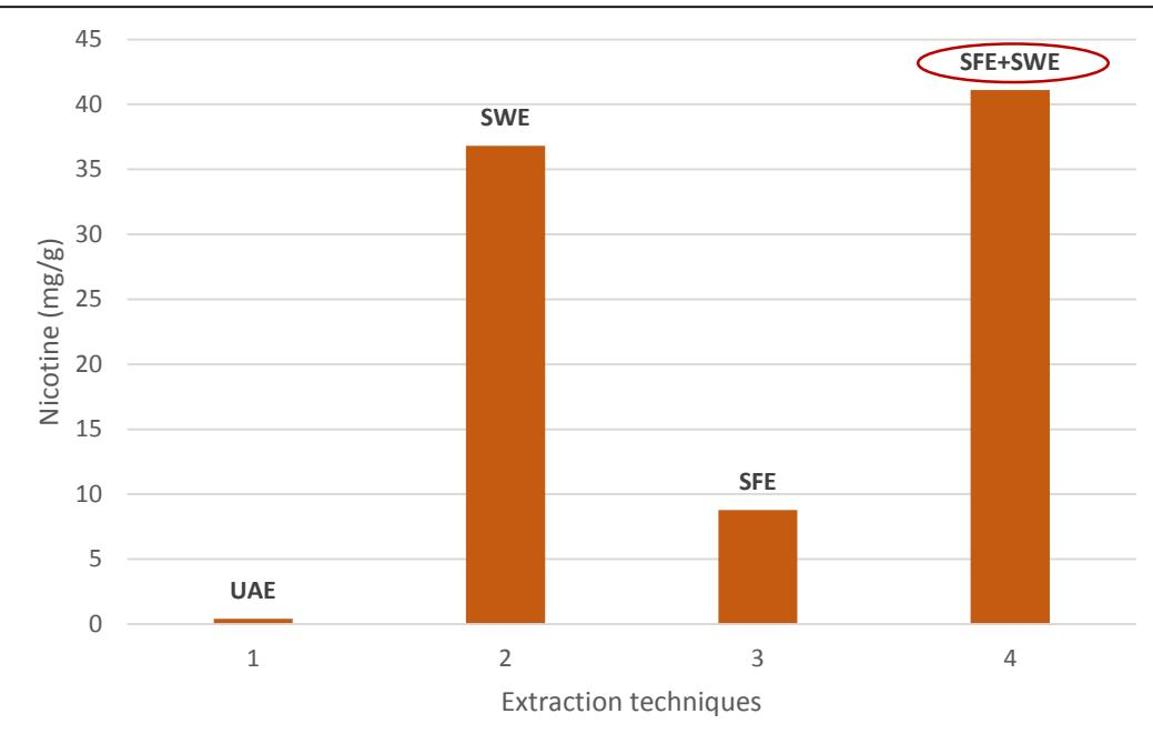
**Figure 8:** Comparison of different methods in extraction of nicotine form tobacco waste
