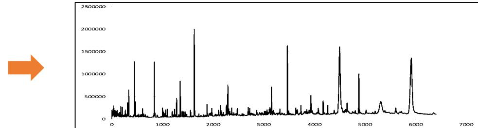
Figure 1: GC-MS midrib chromatogram obtained under UAE condition of 50 °C, 10 min, 10 mL/g
