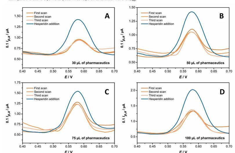
Fig. 4. Differential pulse voltammograms of hesperidin in pharmaceutical samples recorded on ePGE in acetate buffer pH = 5 ( $i_c = 0.1$  mol dm<sup>-3</sup> KCl), scan rate 5 mV/s.  $c_{th}$  (hesperidin) = 3.3 (A), 5.5 (B), 8.2 (C) and 10.9 (D) mmol dm<sup>-3</sup> V(added hesperidin) = 150 μL.
