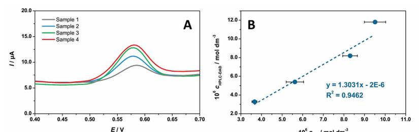
Fig. 3. A) Differential pulse voltammograms of hesperidin in pharmaceutical samples recorded on ePGE in acetate buffer pH = 5 ( $i_c = 0.1$  mol dm<sup>-3</sup> KCl), scan rate 5 mV/s.  $c_{Hesperidin}$  (hesperidin) = 3.3 (sample 1), 5.5 (sample 2), 8.2 (sample 3) and 10.9 (sample 4) μmol dm<sup>-3</sup> and B) Hesperidin concentration ( $c_{HPLC-DAD}$ ) determined with HPLC technique as a function of experimentally determined hesperidin concentration with ePGE ( $c_{exp}$ ).
