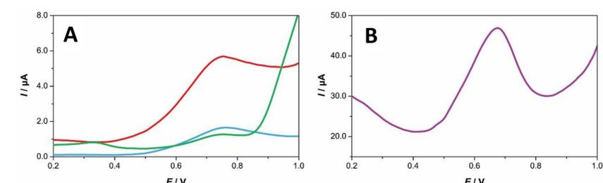
Fig. 1. Differential pulse voltammograms of hesperidin ( $c = 1 \times 10^{-3}$  mol dm<sup>-3</sup>) in phosphate buffer pH = 7.0 ( $i_c = 0.1$  mol dm<sup>-3</sup> KCl) recorded on A) platinum (-), GCE (-) and PGE (-) and B) ePGE (-).
