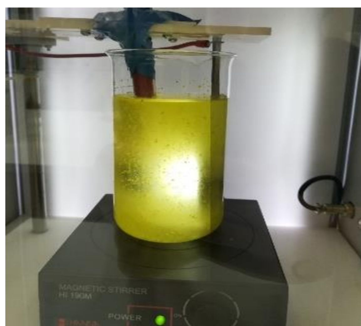
Figure 2. Formation of an electrical discharge between two electrodes in citrus peel extract during HVED treatment
