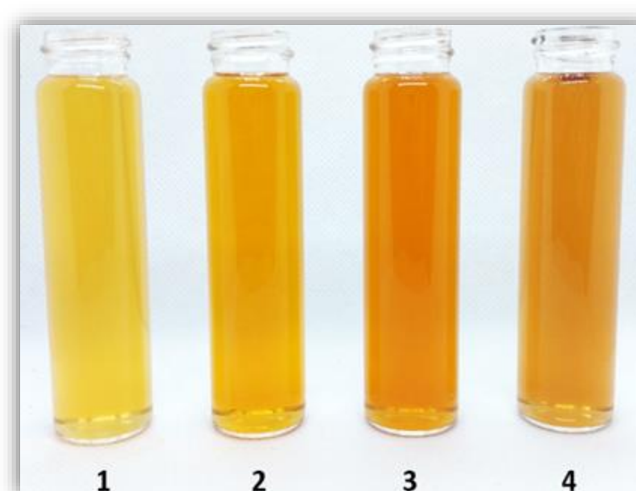
Figure 1: 1-4 extracts after sequential extraction of brown onion skin. Extraction solvent: 96% ethanol (1), 75% ethanol (2), 50% ethanol (3), water (4)
