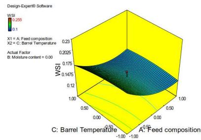
**Fig. 8.** Effect of feed composition and barrel temperature on WSI of lentil and pumpkin incorporated barley based extrudates
