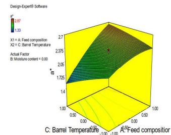
**Fig. 10.** Effect of feed composition and barrel temperature on a\* of lentil and pumpkin incorporated barley extrudates
