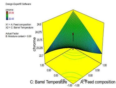
**Fig. 14.** Effect of feed composition and barrel temperature on chrome of lentil and pumpkin incorporated barley based extrudate
