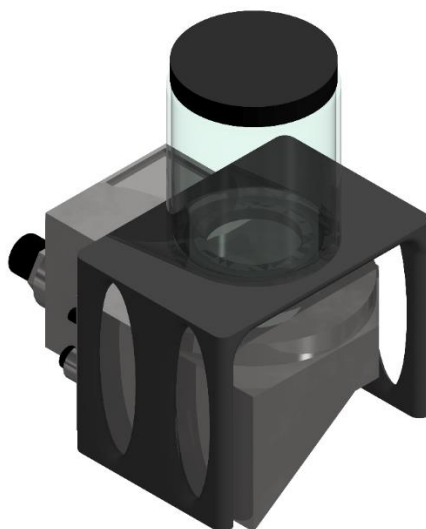
Fig. 1 Schematic view of the experimental setup including contact scan head, sample holder, and sample vessel
