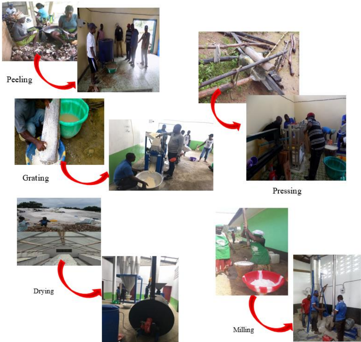
Fig 1. Upscaled cassava processing equipment in Liberia
