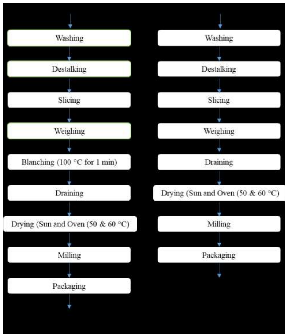
Fig 1. Flowchart for (a) blanched and (b) unblanched vegetable flour processing
