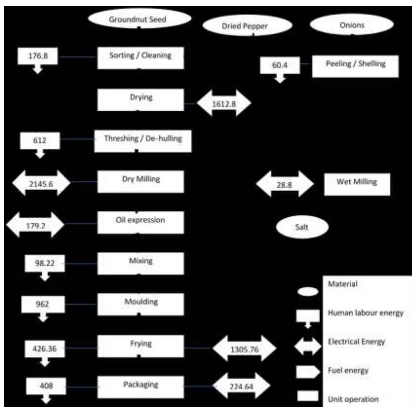
Fig 4. Energy-flow diagram for SMP3
