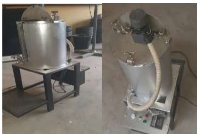
Fig. 3. Pictorial views of the sweetener extractor
