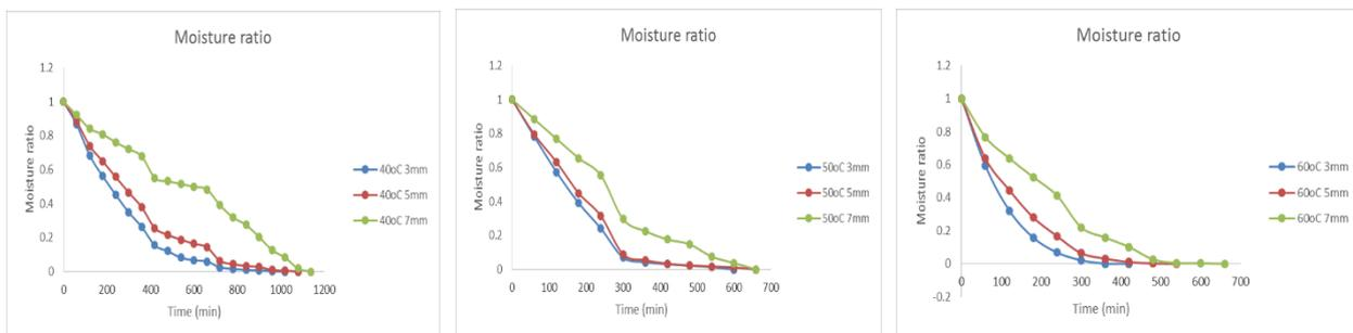
Fig. 2. Graphs of moisture ratio against drying time for turmeric slices
