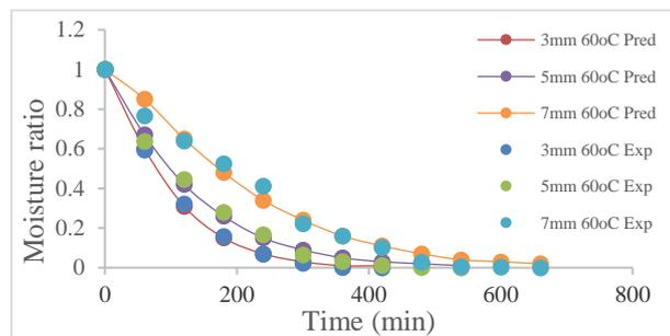
**Fig. 5.** Graph of experimental and predicted values of dimensionless moisture ratio for each thickness at 40 °C, 50 °C, and 60 °C
