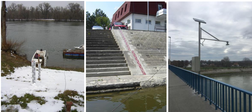
Slika 1. Opažanje vodostaja - običnom letvom, kosom u obaloutvrđi i elektronički, prikladnim sensorom Figure 1. Water level observation - by water level measurement stock (vertical or on the slope of river embankment) and electronically, with a suitable sensor
